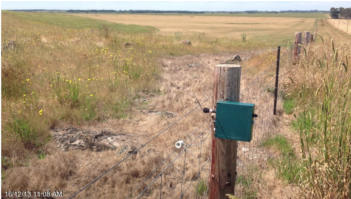
Figure 2: SM2 detector mounted on a fence post
