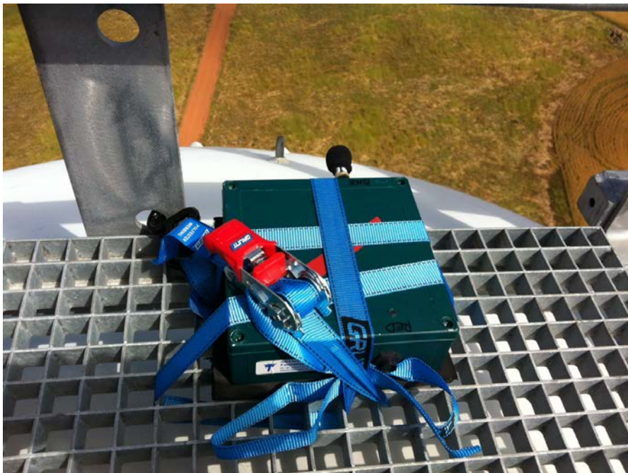
Figure 3: SM2 ultrasonic bat detector mounted on the galvanised mesh platform located on the nacelle of the Goldwind turbines
